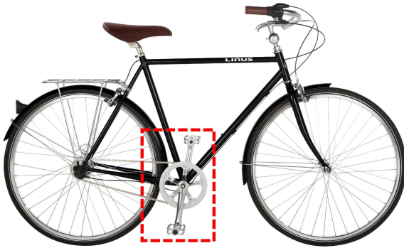
Figure 1: Typical commuter bike with spindle-crank-pedal system highlighted.
